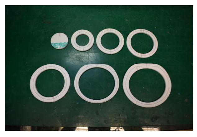
Glue the individual layers together according to the glue line.
