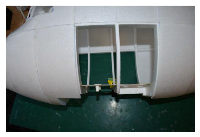
Then cut off the sheeting until the wing fits back on the fuselage with as few gaps as possible.
