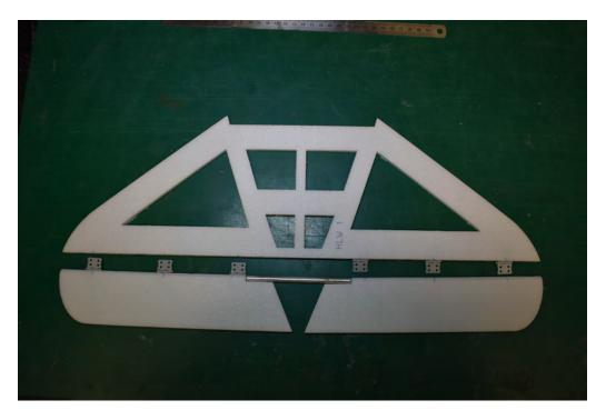
Then put on the 3 mm planking on both sides.
