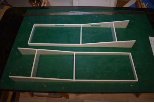
The plywood beam is centered in T1 and glued on a flat surface.
