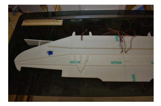
Mount the ailerons using three hinges.
