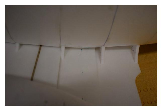
Bend the planking as tightly as possible and glue it to the fuselage and frames. Let it run out at the front according to the course of the planking.
