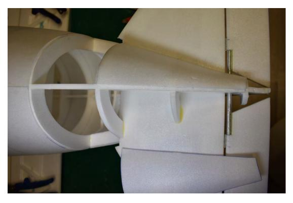
As an example, the servo for the elevator can be placed half open in the planking. So it's better to replace later.
