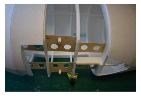
Insert the wing and align it geometrically with the fuselage. Then mark the holes for the two screws.
