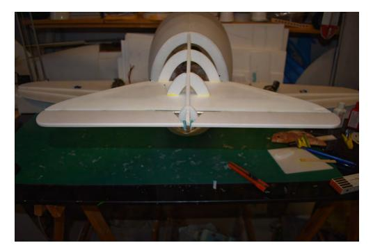
Cut the stringer a bit free so that the elevator can run freely in both directions.
