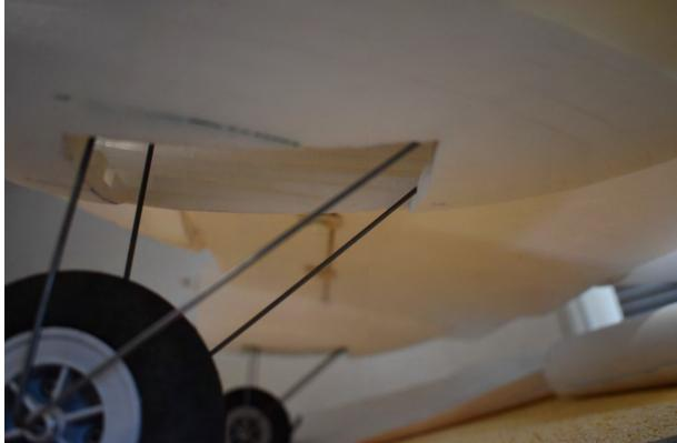
The missing fuselage attachment below the wing can now be glued on.
