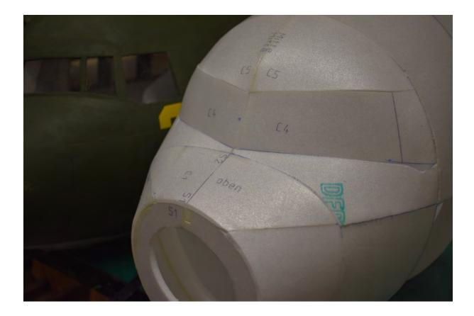
If the windows are to be fitted with clear film/PVC, use the template. The windows can later be closed with 0.3 mm clear PVC film
