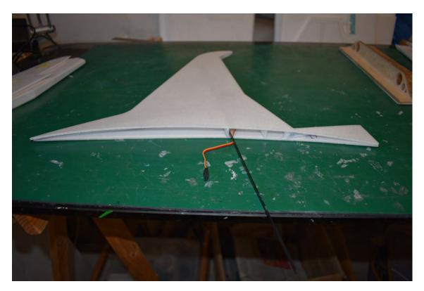
Cut out servo area. Close the rudder immediately and connect it with hinges.
