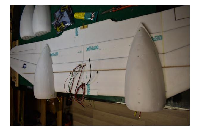
Then glue the lower half of the nacelle on, first transferring the center of the nacelle center from above to the lower wing. (pen mark)
