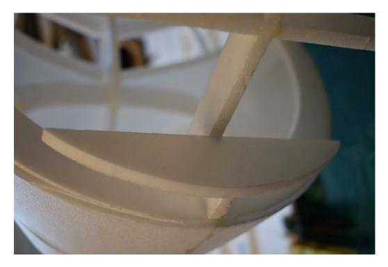
Now the three plankings can be glued on. The stencils have oversize below.
